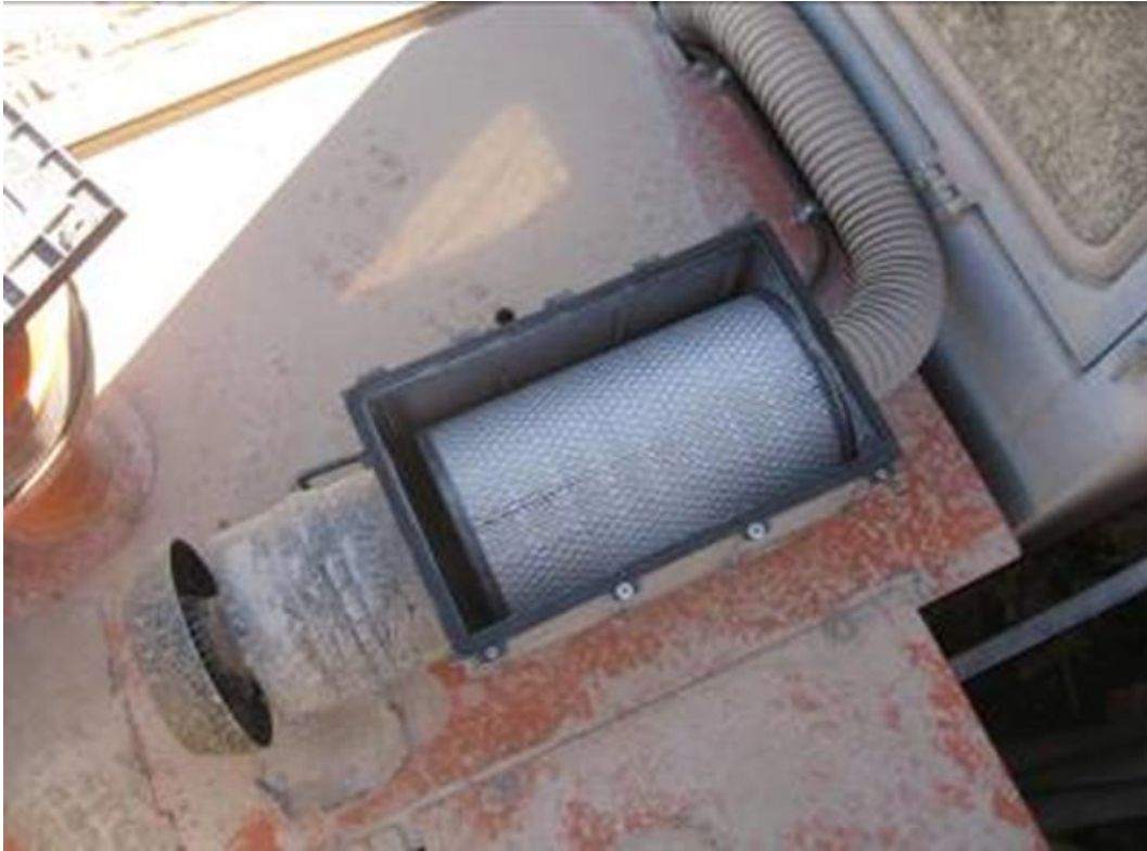
Photo 4.3 Close-up of the RESPA® PFP unit mounted behind the cabin of an Excavator
