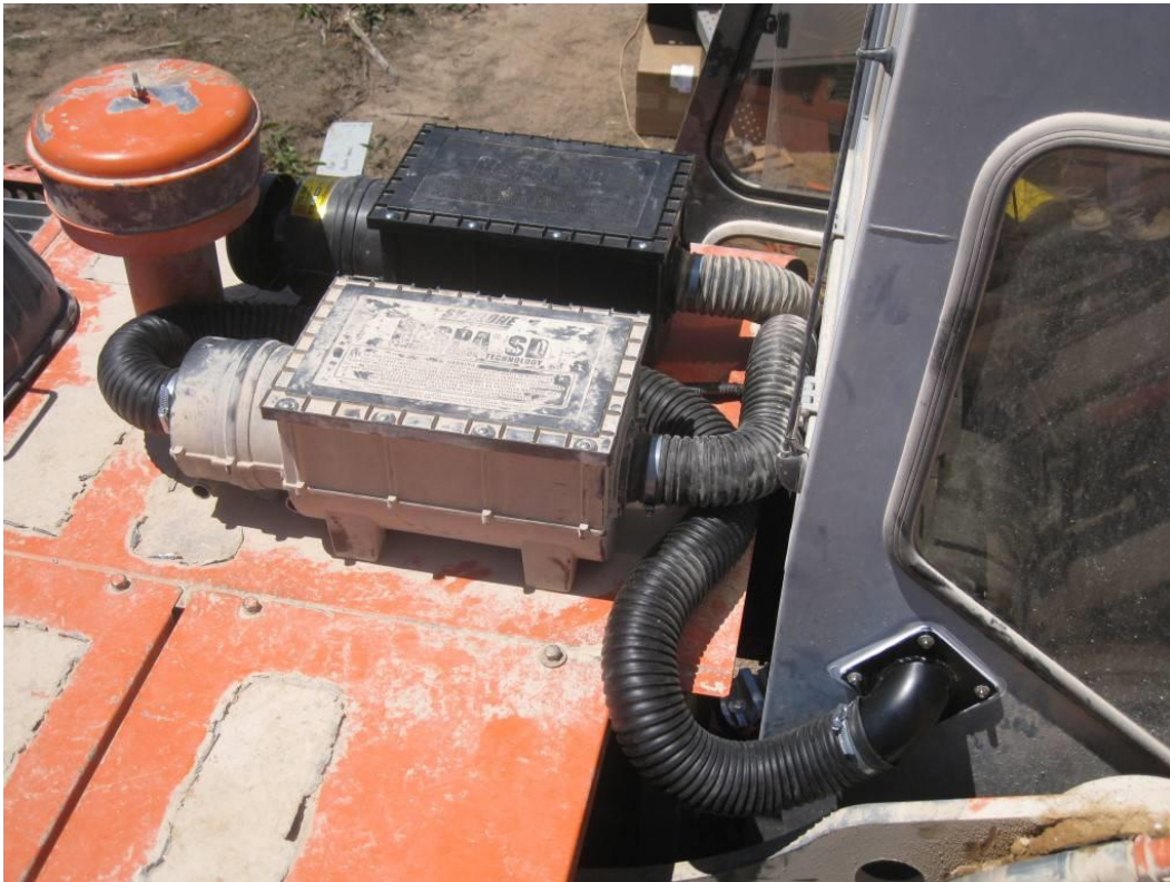
Photo 4.4 Close-up of the RESPA® PFP and second unit mounted behind the cabin of an Excavator.
