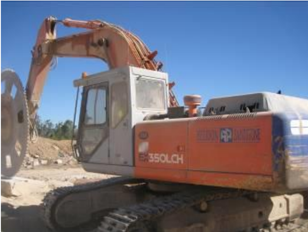
Photo 4.2 RESPA® PFP (new air-cleaning technology) unit mounted behind the cabin of an Excavator.
