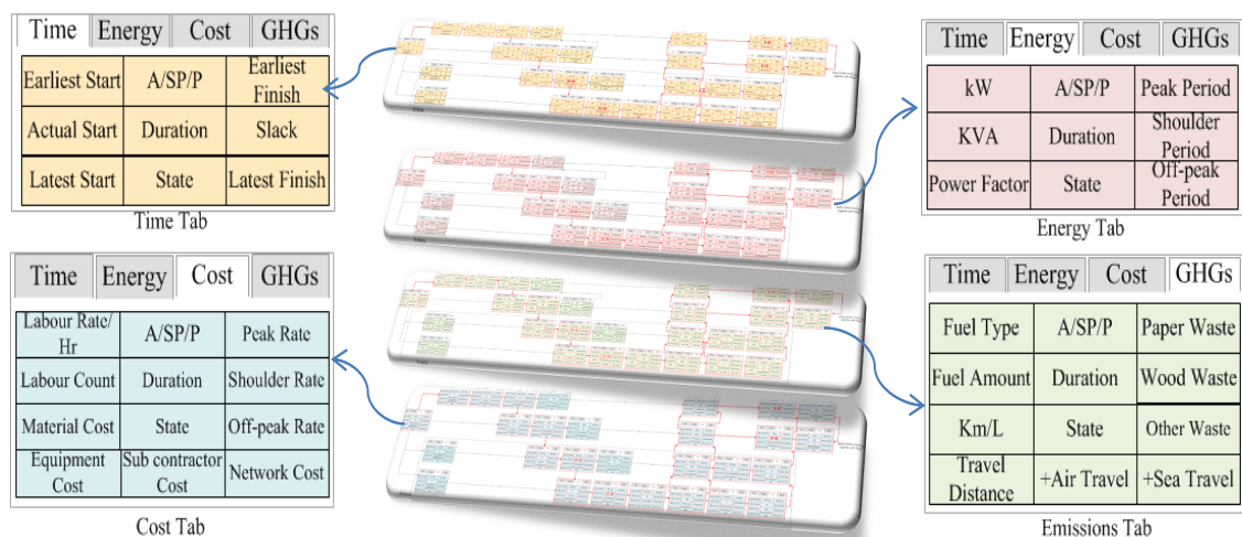
Figure 6.3: Green ABM to model time, energy, cost and GHG profiles of a business process and Time, Energy, Cost and Emissions tabs of a node
