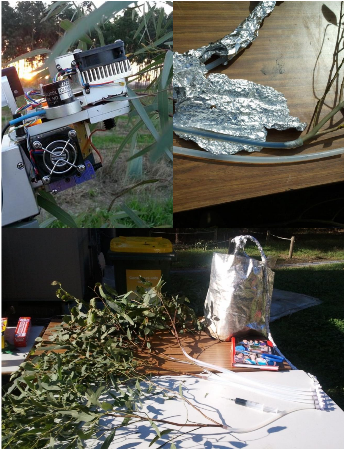
The Li6400 open-flow portable photosynthesis system used for measuring gas exchange (top left) while progressively blocking vessels with india ink (top right) while connected to a KCl reservoir (bottom). Image source: Aimee Bourne, May 2012.
