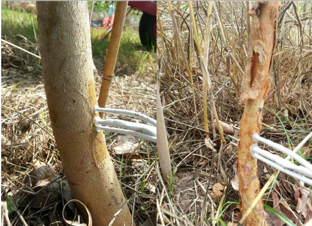
Mixture plantation at planting in November 2011 (top) and sap flow probes in E. tereticornis (left) and E. crebra (right) at the beginning of the study in November 2012. Image source: Aimee Bourne.
