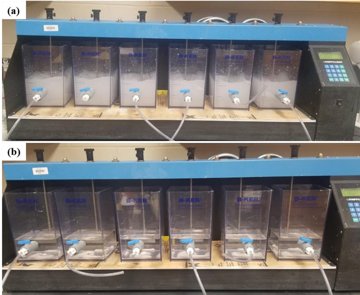
Figure A9.1: Convention jar test apparatus for the coagulation-flocculation process. Images of wastewater (a) before and (b) after the CF process using biopolymer-based flocculant.
