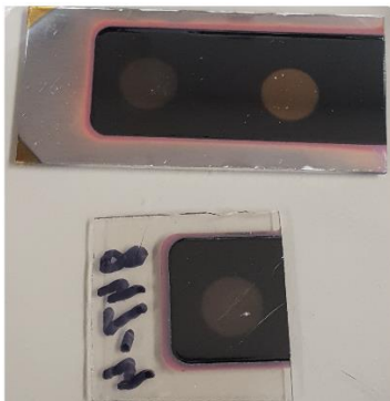
Figure 3.3: Typical 72 \mu\text{m} thick a-Se: 0.3% As + 10 ppm Cl samples. The top sample has an aluminum substrate and the bottom sample has an ITO substrate.
