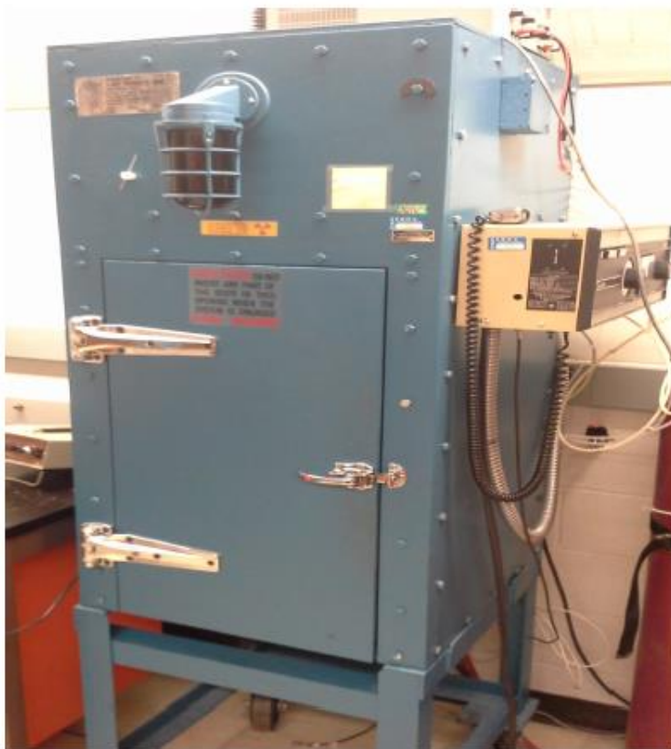
Figure 3.19: Gendex GX-1000 x-ray system and lead lined steel cabinet
