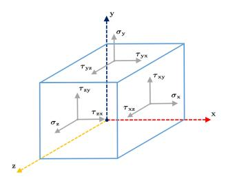
Figure 3.3: Stress Forces on an Infinitesimal Body. The normal stress forces are labelled  $\sigma_x$ ,  $\sigma_y$ , and  $\sigma_z$ . The shear stress forces perpendicular to  $\sigma_x$  are labelled  $\tau_{xy}$  and  $\tau_{xz}$ . Those perpendicular to  $\sigma_y$  are  $\tau_{yx}$  and  $\tau_{yz}$ , and those perpendicular to  $\sigma_z$  are  $\tau_{zx}$  and  $\tau_{zy}$
