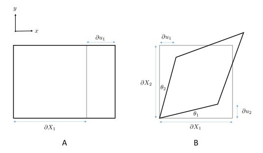
**Figure 3.2:** Measuring Infinitesimal Strain. (A) depicts a cube from a 2D view with an undeformed length  $\partial X_1$  being stretched along the x-axis by  $\partial u_1$ . (B) shows the same cube being sheared instead. The angles  $\theta_1$  and  $\theta_2$  are used to quantify the amount of shearing experienced by the cube relative to its undeformed rest configuration.
