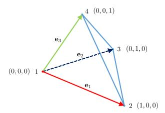
**Figure 3.1:** Tetrahedral Element. The local coordinates  $(\xi_1, \xi_2, \xi_3)$  is provided for each node *i*. The axes of the local coordinate system are individually labeled as  $\mathbf{e}_1$ ,  $\mathbf{e}_2$ , and  $\mathbf{e}_3$ .
