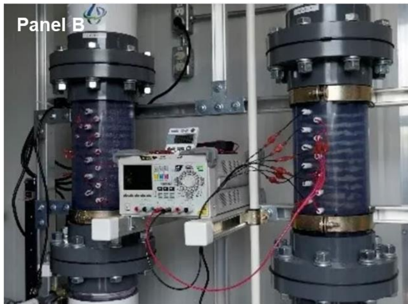
Figure 1-5: Cross section schematic (Panel A) and AOS photo (Panel B) of the current thesis eAOP system. Adapted from BioLargo Water.
