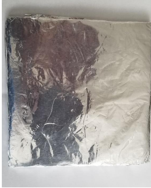
Figure 5-8: Reflector used to measure incident energy
