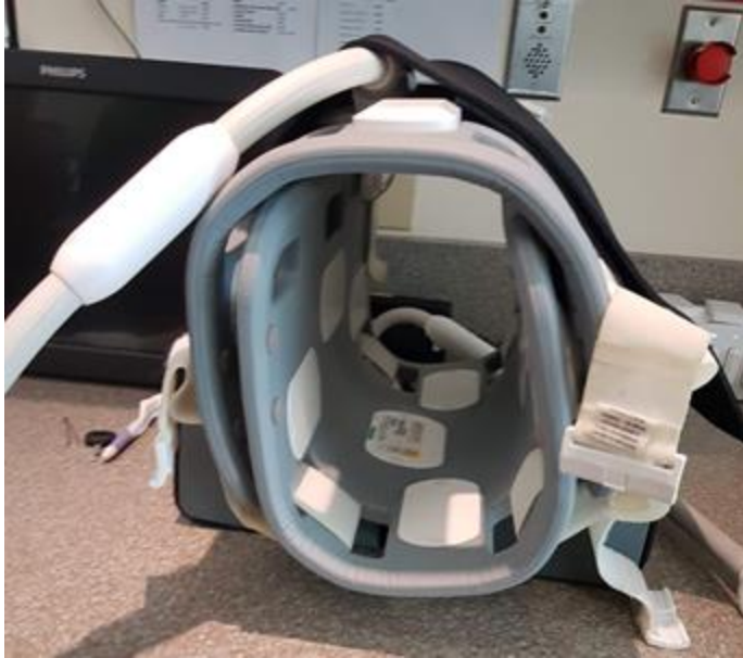
Figure 0-2: Two body RF coils arranged in cage-like form to accommodate knee for MR scanning
