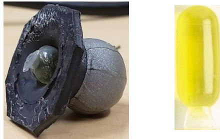
Figure A-6-1: a) Left - MRI marker inserted into the hollow gait marker. B) Right - MRI marker
