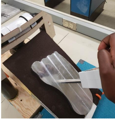
Figure A-2-4: Force gauge being applied with custom-made aluminum foot to mark out angle of tilt on visual cue per individual
