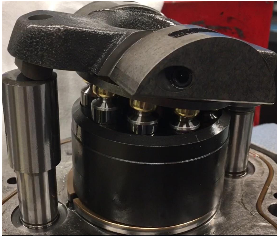
Figure 1.2: Load sensing axial piston pump internal rotating assembly
