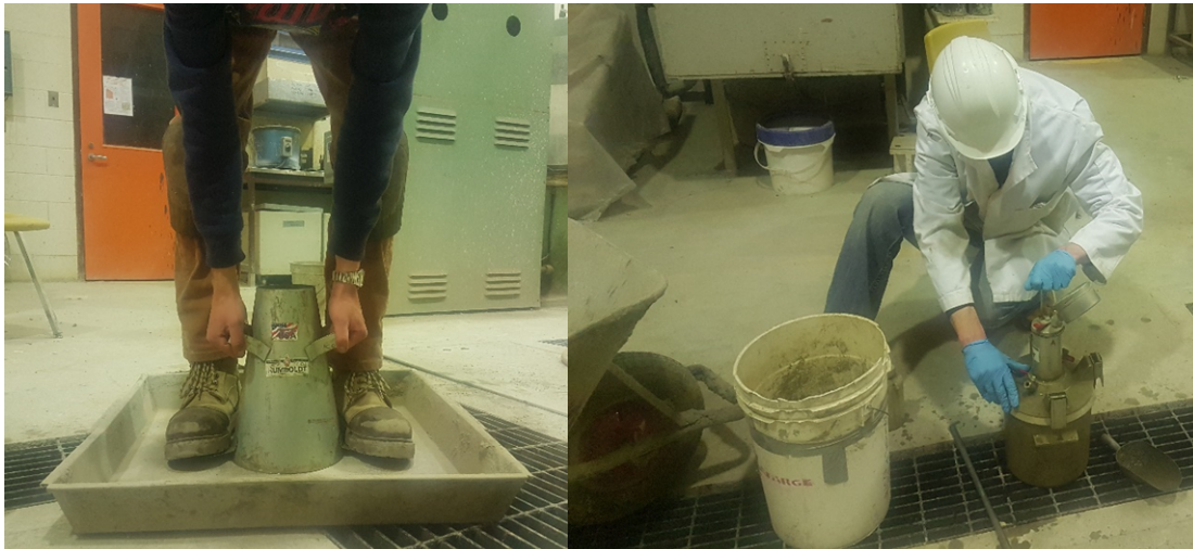
Figure 3.6: Concrete testing: (a) slump, and (b) air content by pressure method
