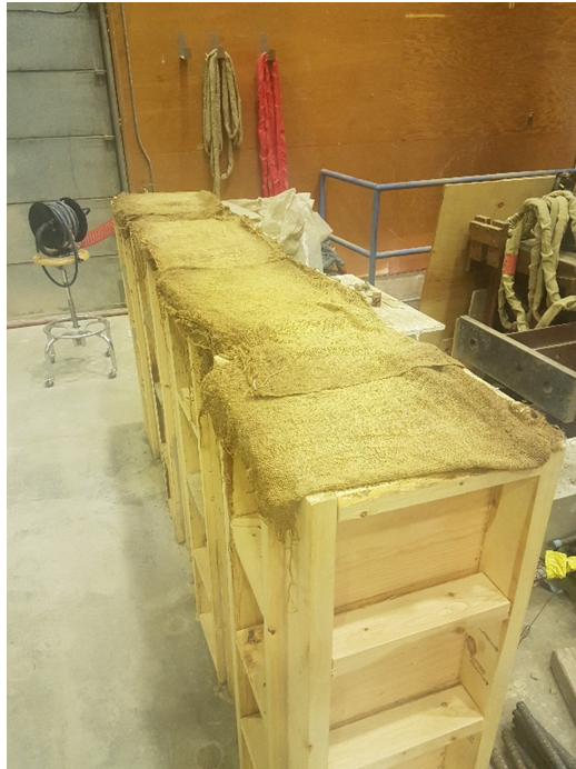
Figure 3.7: Specimens curing with moist burlap
