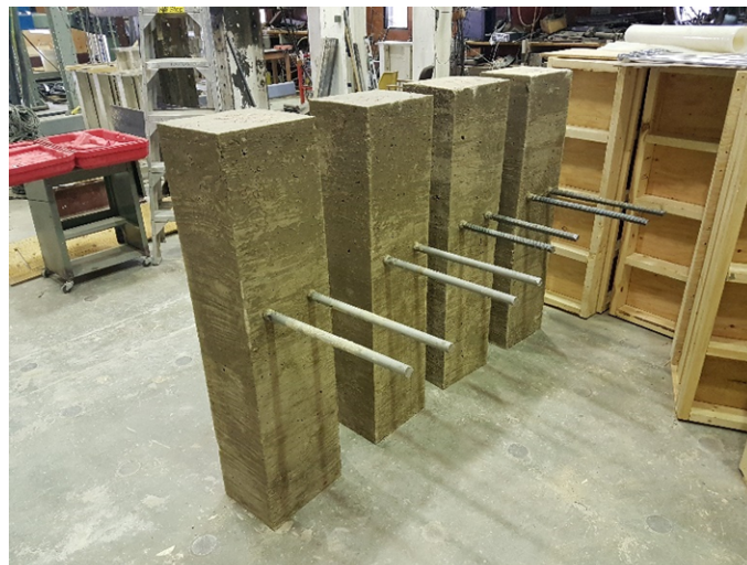
Figure 3.8: Concrete specimens following form removal
