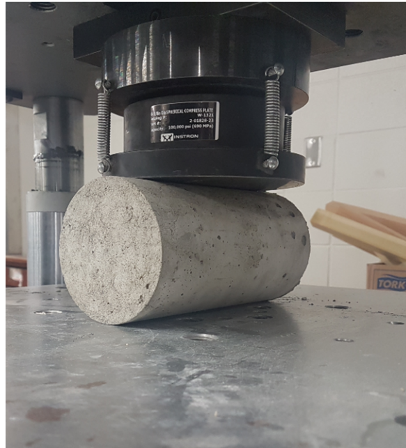
Figure 3.15: Split concrete cylinder testing using the Universal Testing Machine
