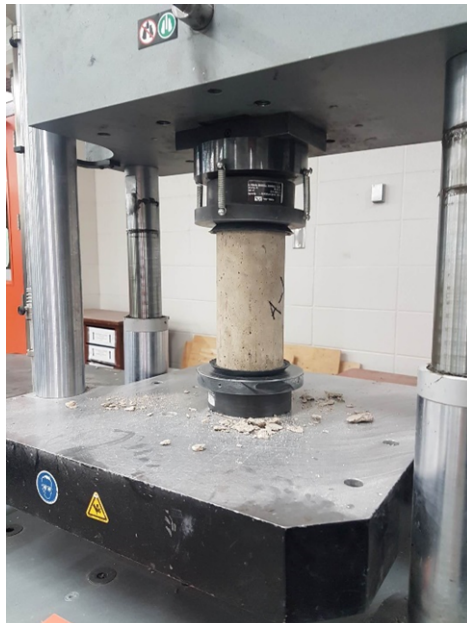
Figure 3.14: Compression concrete cylinder testing using the Universal Testing Machine
