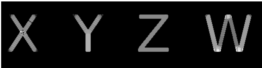
FIGURE 2.11: Stroke Width Transform of Letters X, Y, Z and W
