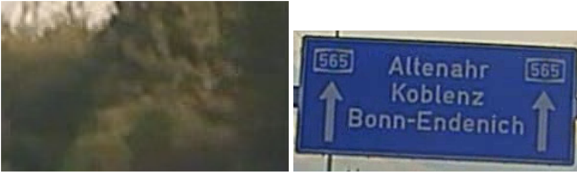
FIGURE 5.3: MPEG Compression artifacts on images from the Fraunhofer Dataset
