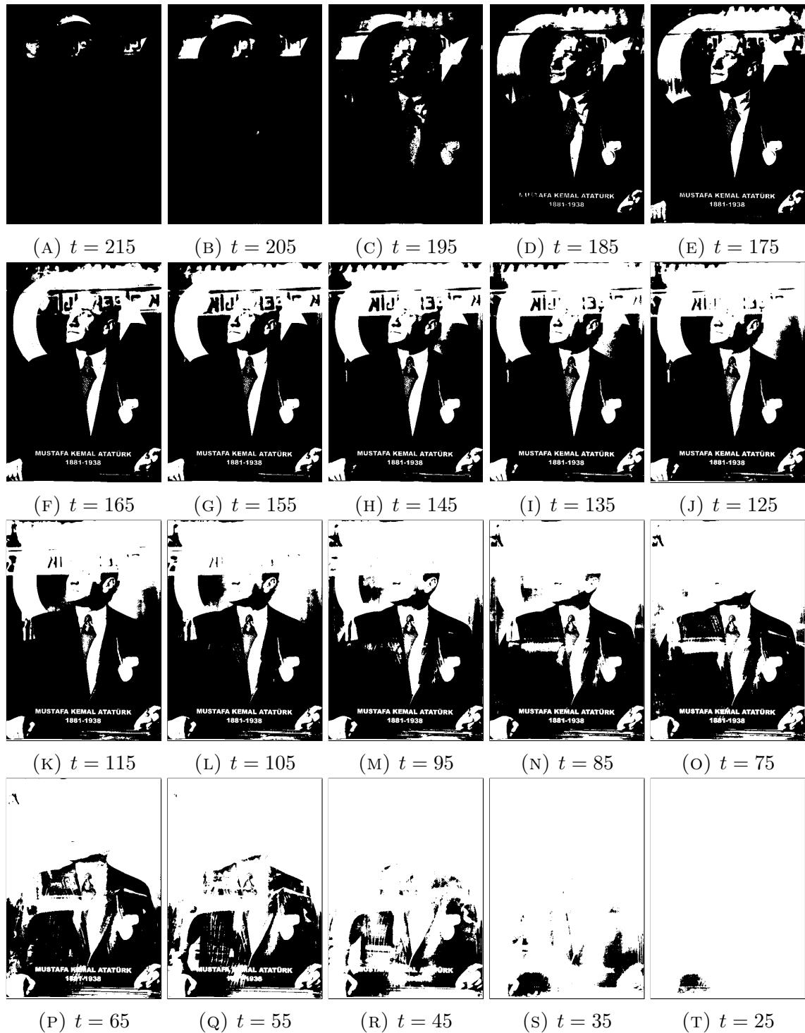
FIGURE 3.9: Thresholding and connected component analysis of an example image. Borders added for clarity
