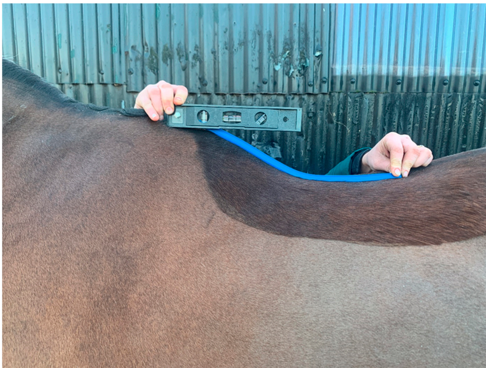
Figure 1. The adapted flexicurve ruler placed on the horse's spine in a sagittal plane to measure thoracolumbar shape. The spirit level is aligned to horizontal and butterfly nut tightened to retain the flexicurve's orientation to the horizontal, before removal to trace sagittal profile.
