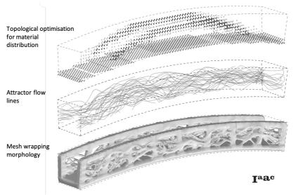
Figure 3.4 Design Development Progress Diagram [46].
