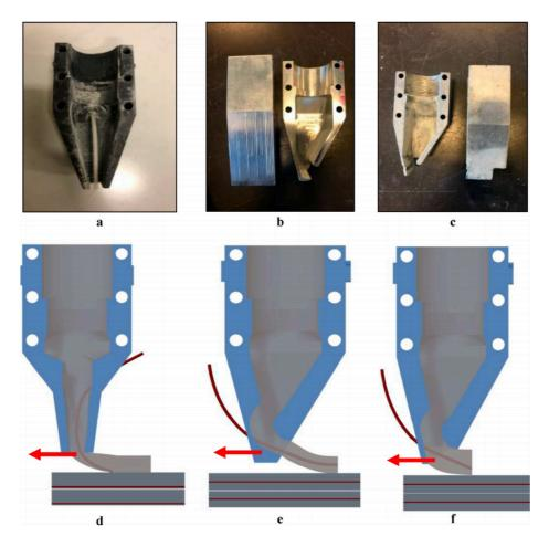
Figure 7.23 Nozzle design and concrete flow [49, p. 229].
