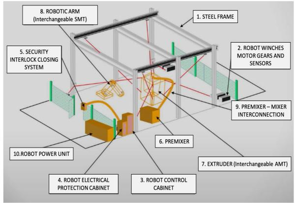
Figure 7.22 All-in-one machine. Elements of the Prototype (AM) [81].
