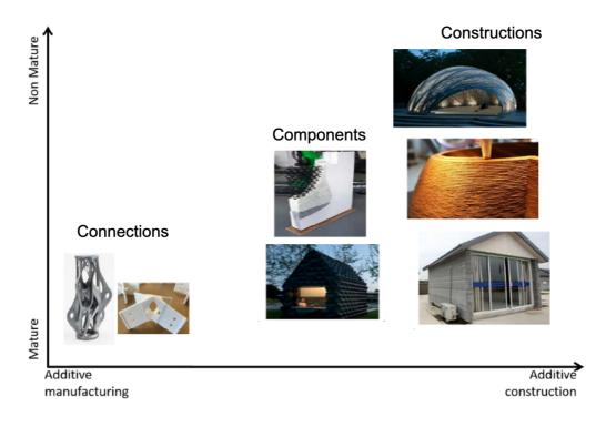
Figure 3.2 Maturity for 3D printing and AM in the Construction Industry [16].
