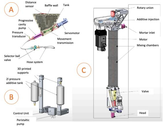
Figure 7.20 A is the Primary Pump, B is the Auxiliary Pump, and C is the Mixer [78].
