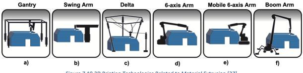
Figure 7.19 3D Printing Technologies Related to Material Extrusion [27].
