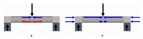
Figure 7.32 Principle of pre-stress applied to a structure loaded in bending. (a): no pre-stress, only bending, (b): pre-stress and bending: the tensile stress in the bottom of the structure is eliminated [49, p. 224].
