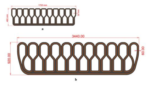
Figure 7.33 Print paths of the 1:2 scale model for testing (a) and the actual bridge section (b). The optimised pattern of the latter with regard to the former saves 4 percent of print path length [49, p. 226].
