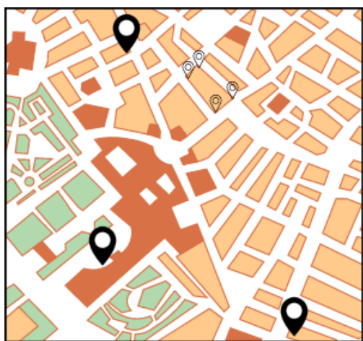
Point represents a specific GPS coordinate on a map Polygon markers. This shape contains a set of GPS coordinates based on the shape of the polygon
