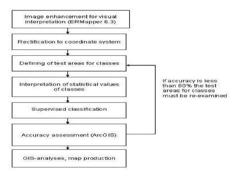
Fig. 4. The image processing procedure.
