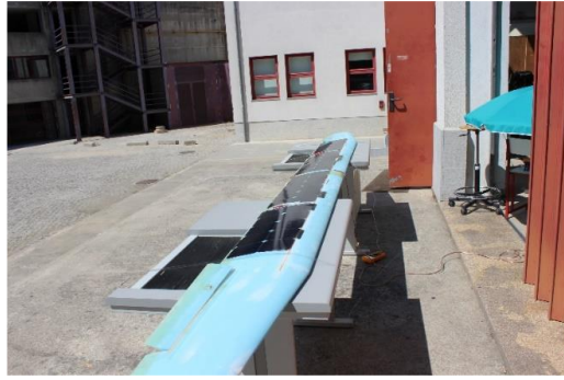
Figure 2 - Sousa's Solar module attached to the LEEUAV wing prototype [5]
