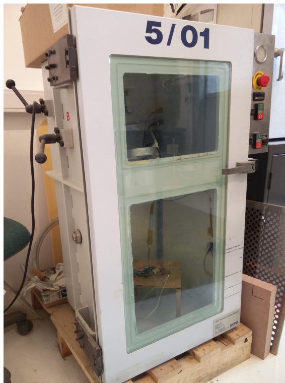
Figure B.4: Vacuum chamber used to perform the experimental test. It provided the controlled environment desired. The convection heat transfer was minimized.
