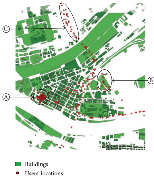
FIGURE 11: An example of one user's GPS locations projected on the geographic entities layer of Pittsburgh; (A) stationary activity, (B) moving activity, and (C) moves.
