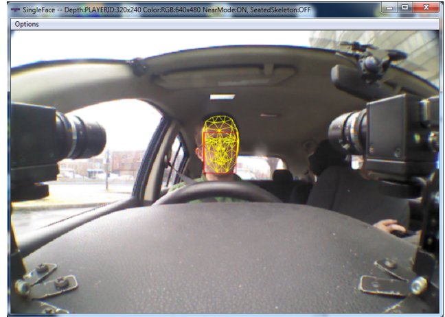
Figure 2 Kinect camera and head recognition system installed in the LiSA lab 1 .
