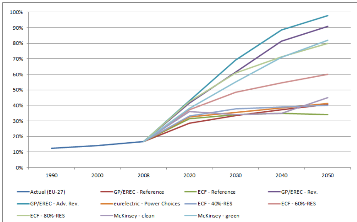
Figure 4 Development of the share of renewable energy sources in electricity generation (including net imports) in the different scenarios
