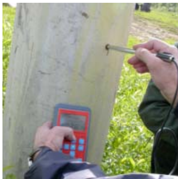
Photo 6: Measurement by means of thermo-anemometer.
