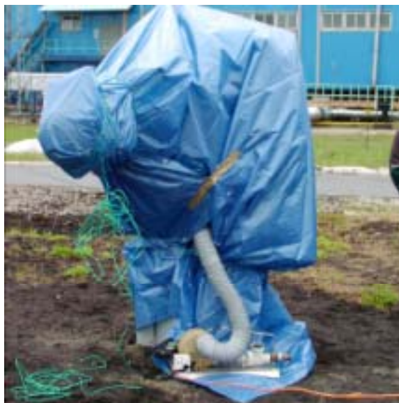
Photo 10: Volume measurement at a gate valve Uchta, June 2003.
