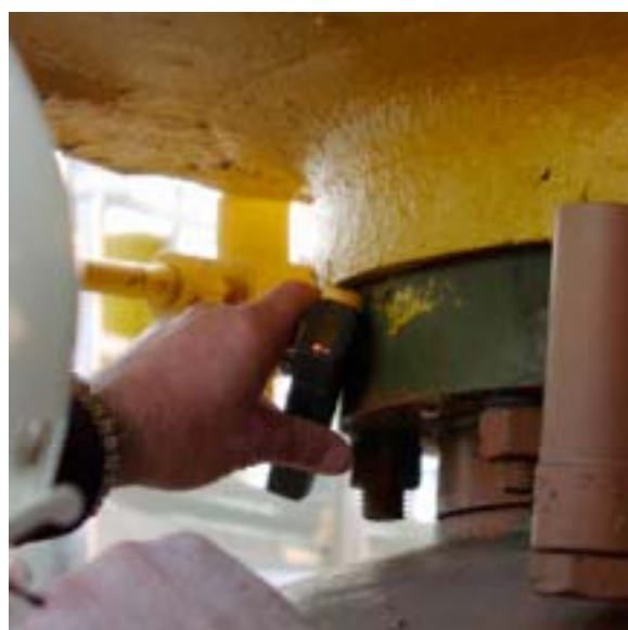
Photo 7: Valve screening with Jansky detector.
