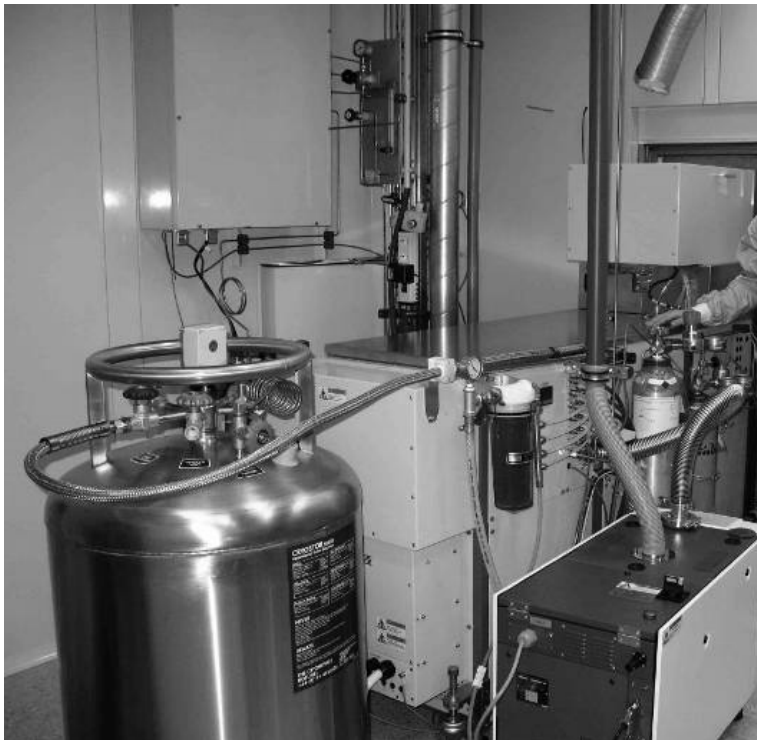
Figure 3.3: Oxford Plasmalab 100 equipment used in MEMS Lab in MTA TTK MFA
