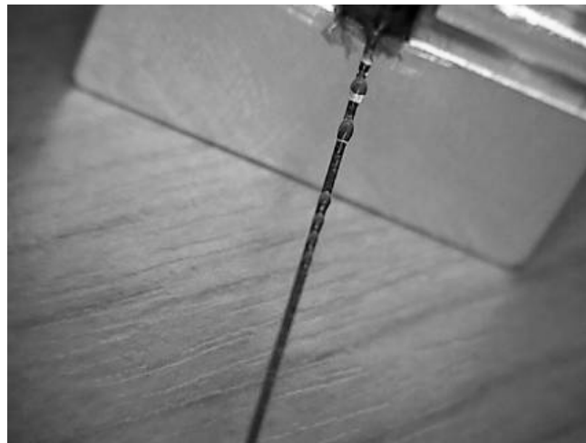
Figure 4.39: Typical leakage through poly-silicon orifice above the critical pressure.
