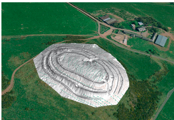
Fig. 8. The 2005 hachure drawing draped over the dGPS DTM of Castlelaw Fort, set in the context of the Getmapping landscape photography. The drawing shows the 18 th /19 th century cultivation furrows cutting across the central area of the fort. (©Crown Copyright. All rights reserved. Background images and landscape height model data copyright of Getmapping® and Intermap®)
