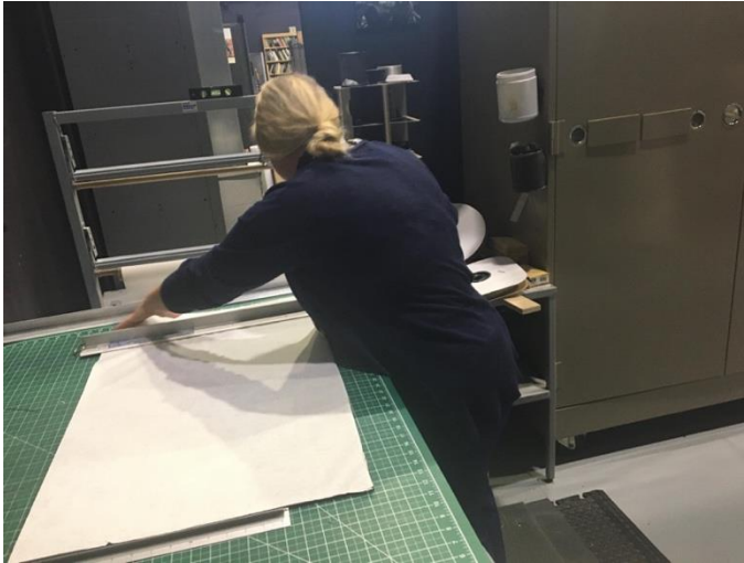
Figure 1 shows Heil cutting the adhesive paper to fit the size of the foam board.
