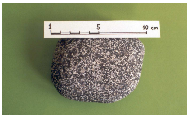
Fig. 15. Classical textbook gabbro from the Samail ophiolite. Black and white minerals have about the same size and are distributed equally ("isotropic" gabbro) throughout the rock.
