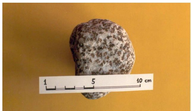
Fig. 16. Though this rock resembles granite, it belongs to the gabbro family, because the white minerals are not quartz, but calcic plagioclase feldspars. The originally black iron-rich minerals have "rusted", that is have oxidized. This specimen is a water-worn pebble from the Wadi al Khod.
