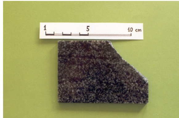
Fig. 14. Cut and polished slab from Khor Fakkan which shows a slight "layering" of the black minerals.
