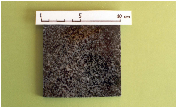
Fig. 7 Gabbro is the classic textbook type. All over the world it is used for decorative floor – and wall tiles. Oman has enormous deposits of this "isotropic" gabbro, but it is not yet mined. This cut and polished tile from the Samail ophiolite was tested at the Department of Petroleum, Mining Engineering, College of Engineering/Sultan Qabus University, and was found to be of excellent quality, and suitable for sculpting purposes.
