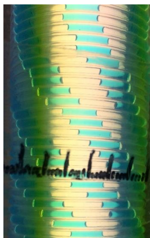
Figure 4.10: Gas-liquid slug flow formed inside the reaction capillary.
