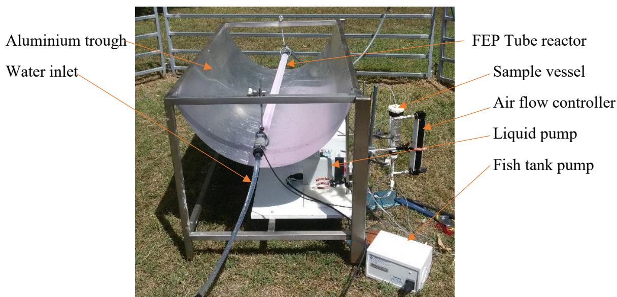
Figure 3.3: In-house parabolic trough concentrating solar reactor.
