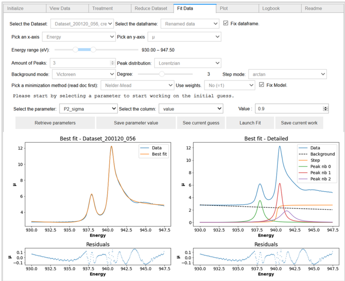
Figure 12: Screenshot of the THORONDOR peak-fitting toolbox. In the graph on the left is reported the comparison between the experimental spectrum and the best fit referring to a \text{Cu}_2\text{O} sample, while on the right are showed all the optimized profiles. The associated R-factor, quantifying the misfit among the experiment and the best fit is R_{XS}^2(\%) = 0.15\% .
