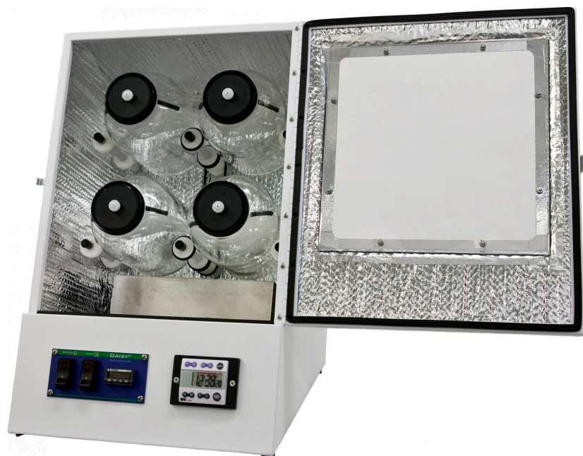
Figure 1. The Daisy II incubator (Ankom Technology Corporation Fairport, New York, NY, USA).
