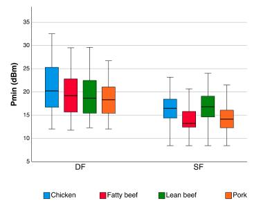
**Figure 5.** Comparison of the Single Frequency (SF) and Dual Frequency (DF) tag types on four meat types when detection is performed in the UHF band. The data are expressed as the minimum power required to activate the tags ( $P_{min}$  (dBm)) on a box-plot graph. The tag types are compared in the 2.5–18.75 mm range of distances.
