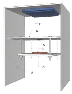
**Figure 2.** UHF test bench: (**A**) low-density polystyrene box, (**B**) central fixed shelf, (**C**) UHF tag, (**D**) adjustable platform, (**E**) meat sample and (**F**) UHF panel antenna.
