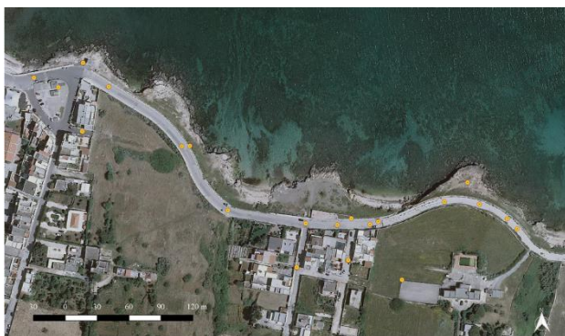
Figure 1. WMS Service of SIT Puglia © Orthophoto 2016. Representation of the 30 GCP/CP distribution in the scenario by means of orange dots.
