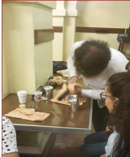
Fig. 4. Construction of low-cost Leyden jars with plastic cups and aluminium foils.
