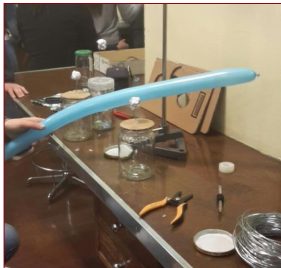
Fig. 5. Electroscopes with glass jars and their covers.
