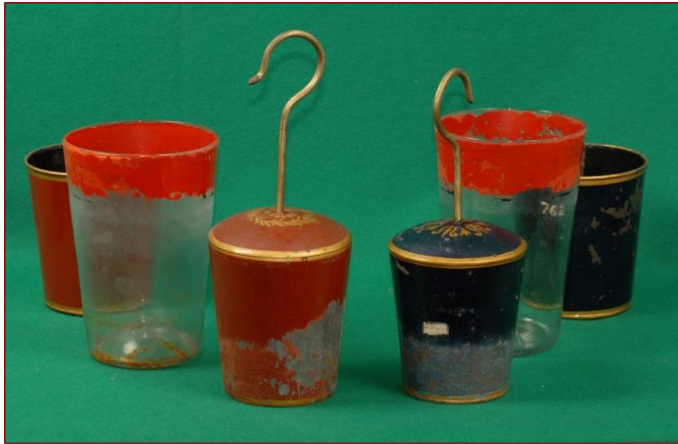
Fig. 3. Two sets of early 1800s dissectible Leyden jars preserved by the Museum of Physics of the University of Turin (inv. n.: 761).
