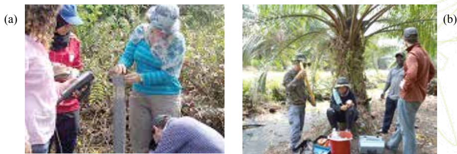
Measurement of dissolved organic carbon in groundwater from (a) piezometer and (b) drainage channels in an oil palm plantation in the study area
