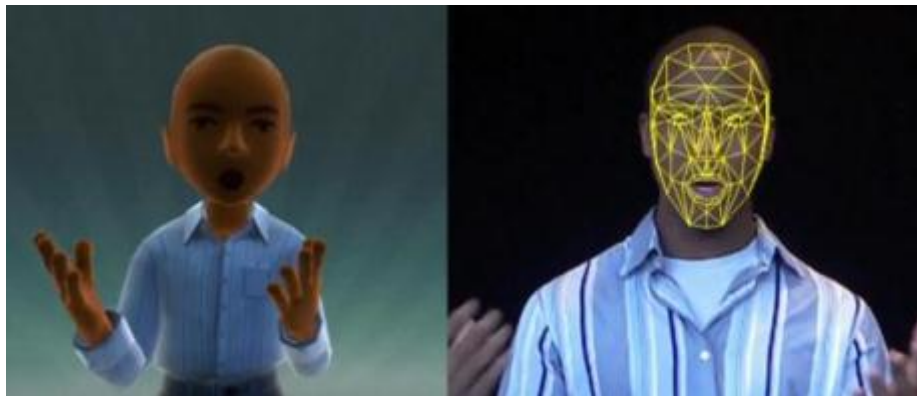
Figure 2: Right image : face and emotion tracking, Left image : emotion reproduction on an avatar. Extracted from [MIC_AVA12].
