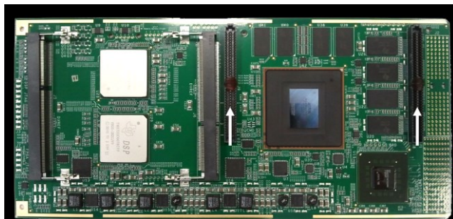
Fig. 2. The Front-End board. Top: Block-diagram; Bottom: view of the upper board side showing the FPGA (on the right) and the two DSPs. The high power TX and T/R switch board is hosted by the high-speed connectors indicated by white arrows.
