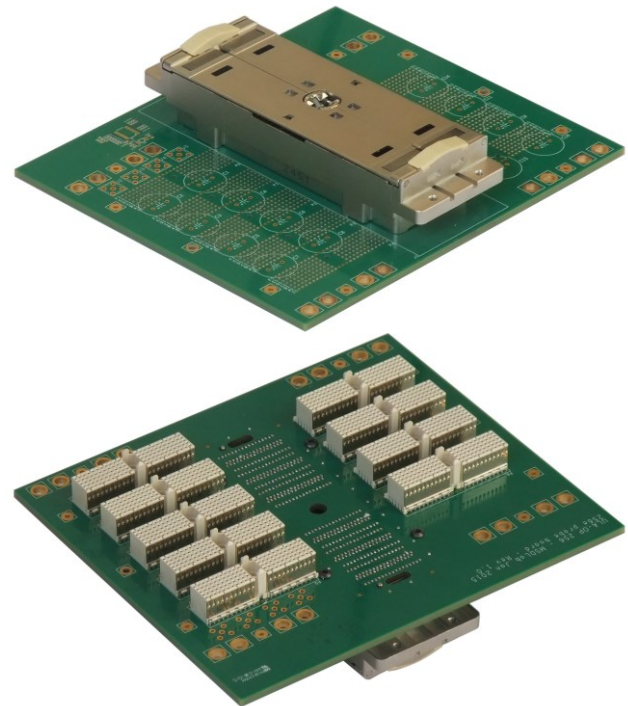
Fig. 3. Probe adapter module for 256-element probes. Top: the shielded DLP408R connector; bottom: the shielded connectors that mate with the system backplane.
