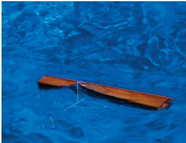
Figure 10. 1/200th scale ark model showing high wave action for the heavier weight model. The white lines demark the trough and peak of a wave. In this picture, the size is 7.1 inches relating to a 118ft wave. The ark did not tip over in any of the circumstances.
