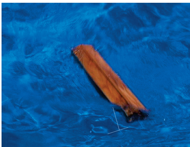
Figure 11. 1/200th scale ark model showing high wave action for the heavier weight model. The white lines demark the trough and peak of a wave. In this picture, the size is 6.17 inches relating to a 112ft wave. The ark did not tip over in any of the circumstances.
