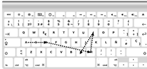
Figure 2: A drawmetric profile of the word “admin” overlaying a standard QWERTY keyboard.
