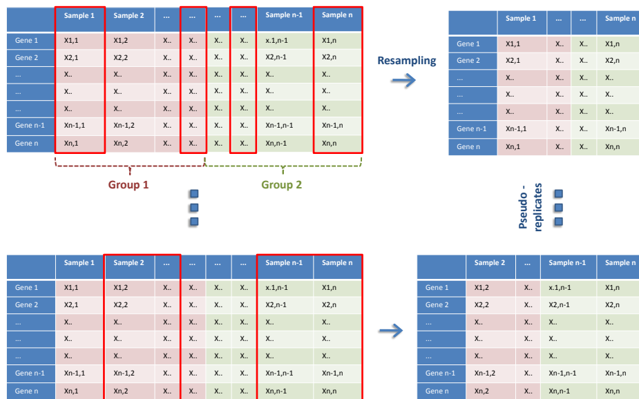
Figure 4.17: The microarray gene expression data are perturbed by jackknife resampling. Thereby samples are drawn without replacement from the gene expression matrix. A 50% jackknife is applied, drawing randomly 50% of the samples in the gene expression matrix from each group. This produces a different gene expression set each time.
