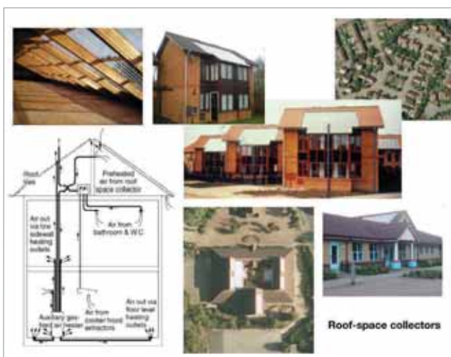
Figure 5: Roof-space solar collector diagram showing (clockwise from bottom left) operation of a domestic system; interior view of glazed loft space; exterior view of a domestic system, aerial view of a group of domestic systems; staggered row of domestic systems; system on a school building (Norton, and Waterfield, 1990); aerial view of system on a school building.
