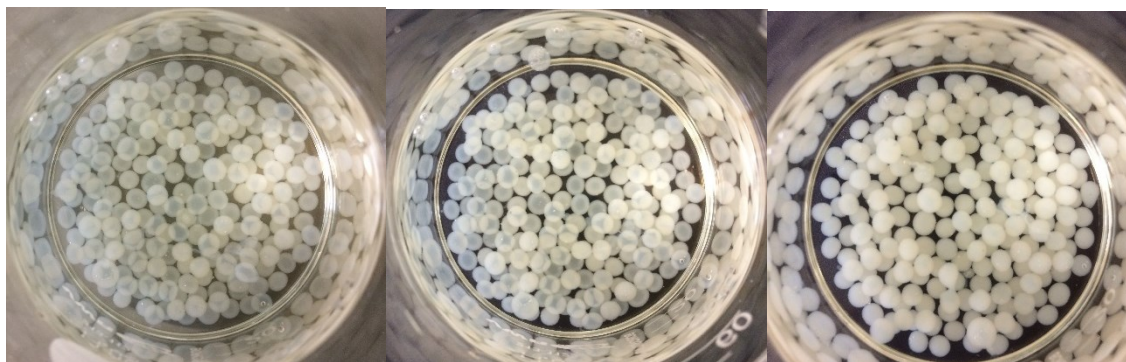
Figure 6.6: The curing of calcium alginate beads with time in \text{CaCl}_2 solution. With increased incubation (15mins, 30mins and 60mins depicted in the images from left to right), the beads turned from clear to opaque due to hardening. All the enzyme entrapped, and non-enzyme entrapped calcium alginate beads, were left to cure in \text{CaCl}_2 solution for 60mins before further washing and storage.
