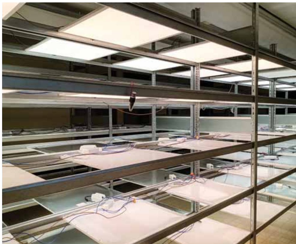
Testing facilities at Laborelec in Belgium where the LED luminaire panels are currently being tested.
