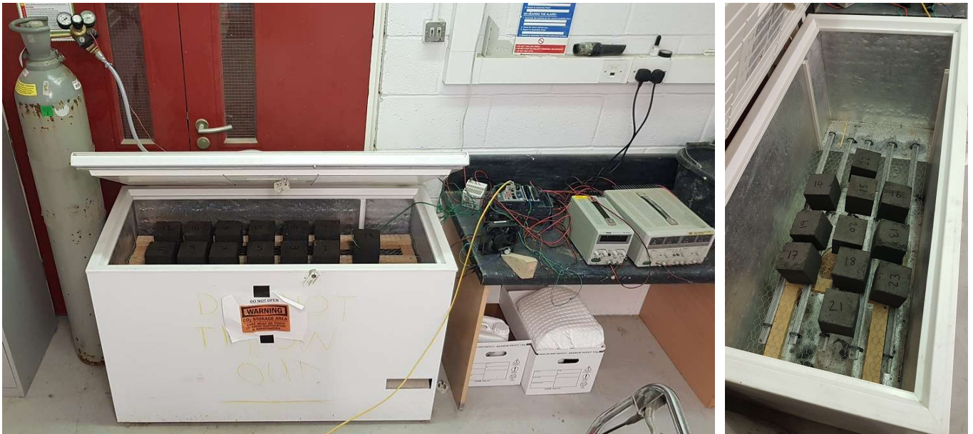
Figure 1. Accelerated carbonation curing chamber
