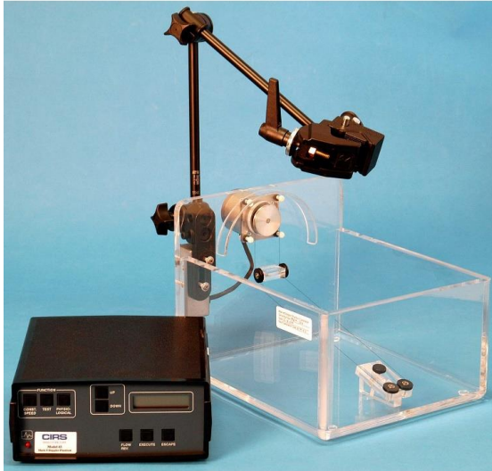
Figure 3.6: A CIRS string phantom consisting of a linear motor and a string with a strong acoustic response
