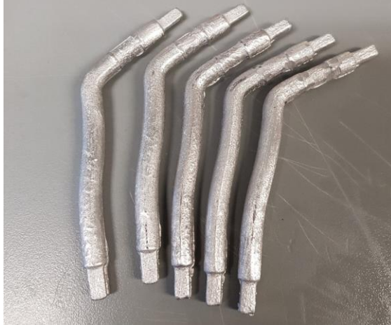
Figure 4.3: Lumen moulds made of low melting alloy. The vessel mimicking material was moulded around these inserts to produce an anatomically realistic vessel lumen. The low melting alloy could be removed later by placing the phantom in a water bath at 60°C.
