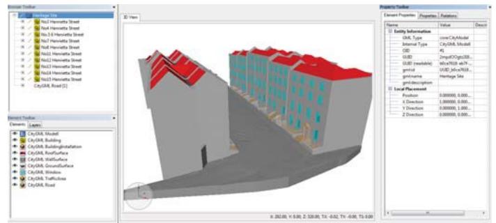
Figure 3: CityGML Model Showing Semantic Classes (Dore and Murphy 2012)
