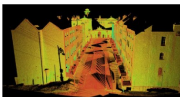
Figure 1: Laser Scan Survey of Henrietta Street
