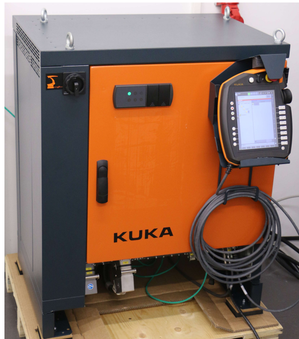
Figure 2.2.: KUKA KRC-4 robot controller with KUKA KCP teach pendant
