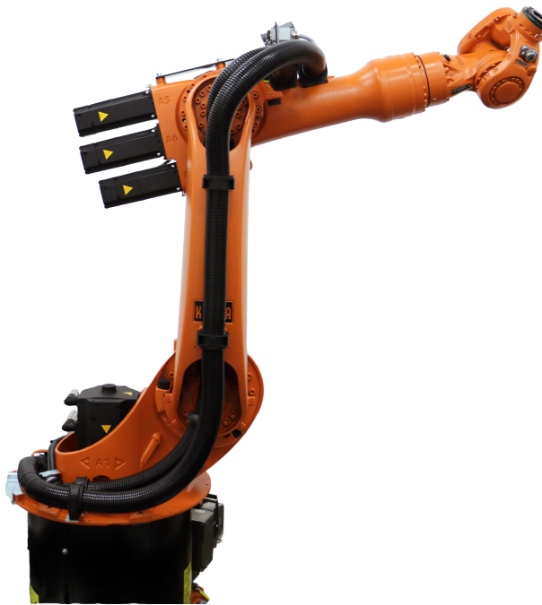
Figure 2.1.: KUKA KR-16, a typical industrial robot with six revolute joints.
