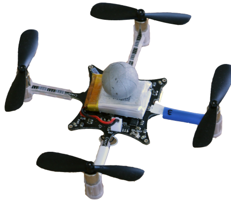
Figure 11.8.: Crazyflie miniature quadcopter with infrared reflecting marker for position tracking
