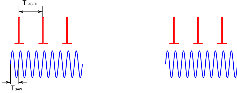
Figure 3.4: Illustration of phase locked mode. The SAW and the laser pulses are synchronized having a fixed relative phase. Because of the limited repetition rate of the laser f_L , the frequency of the SAW f_{SAW} is a multiple of the laser trigger rate.
