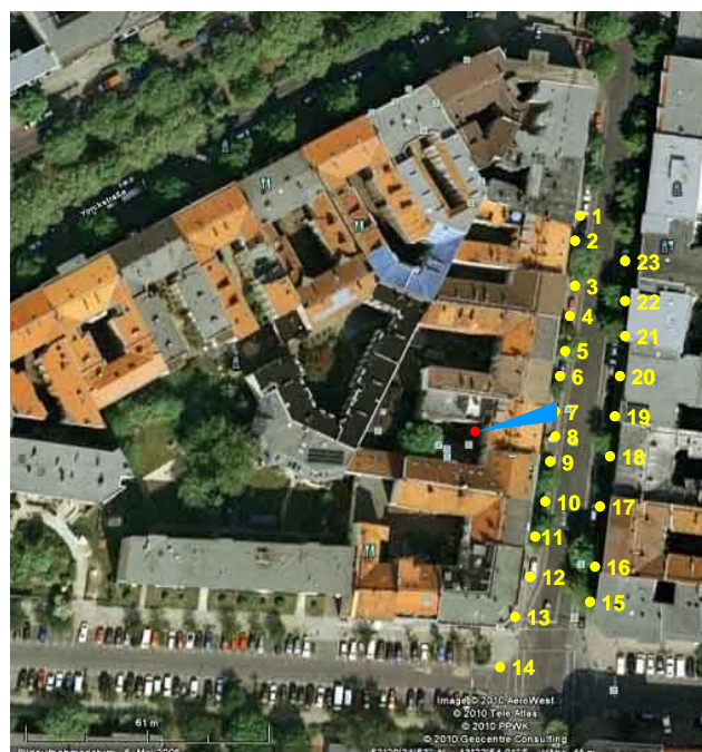
Figure 6. Coverage of the IEEE802.15.4-2006 2.4GHz module with 5 dBm transmit power and 250 kbps. Map source Google Earth.
