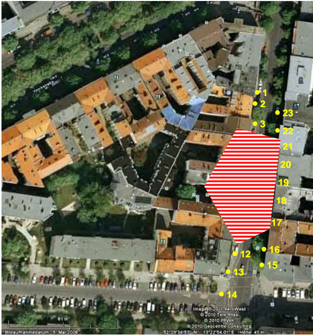
Figure 7. Coverage IEEE802.15.4-2006 PSSS 868MHz "TRx154b_Eval" module 0 dBm Tx power and 250 kbps data rate. Map source Google Earth.
