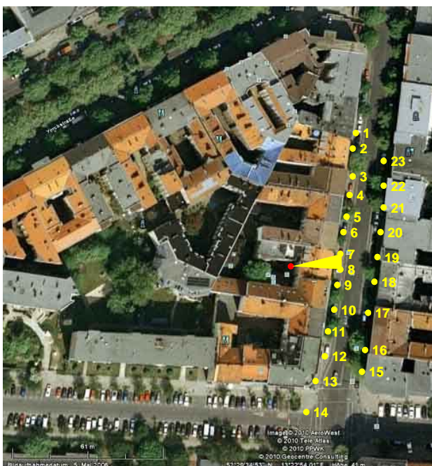
Figure 4. Coverage of the 868MHz Wireless M-Bus module, 0 dBm transmit power, 16.38 kbps. Map source Google Earth.
