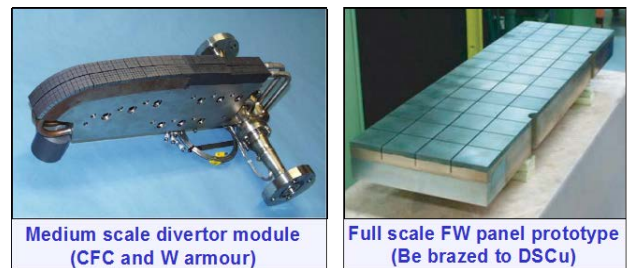
Fig. 7 Medium scale mock-up for the divertor and the first wall of ITER
