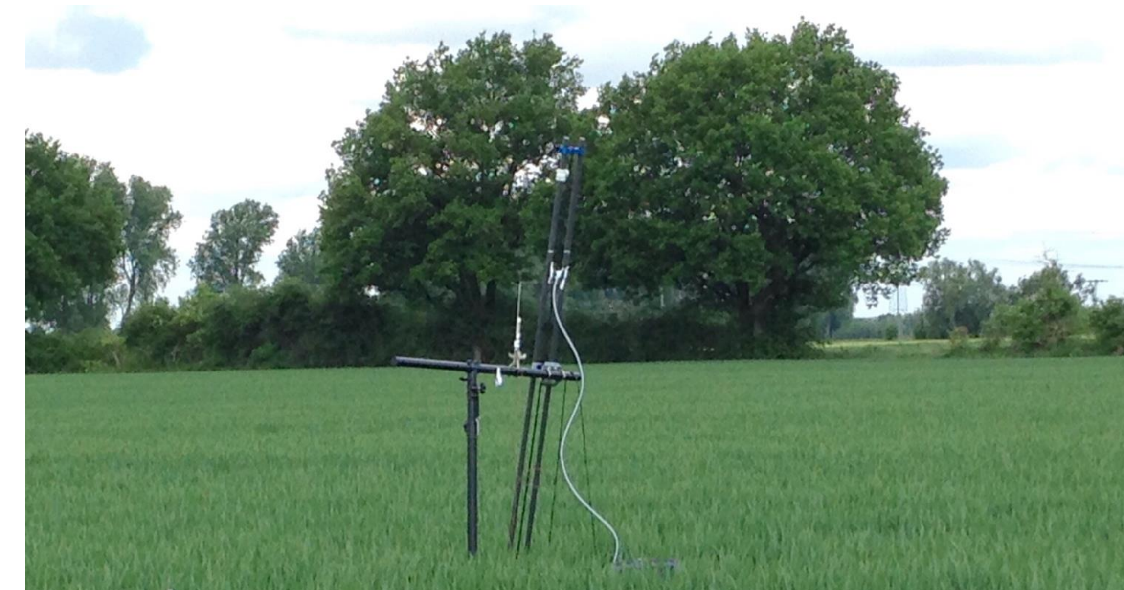
Fig. 2: Profile-measurement system operating at the test site Selhausen in winter wheat (May 2015).
