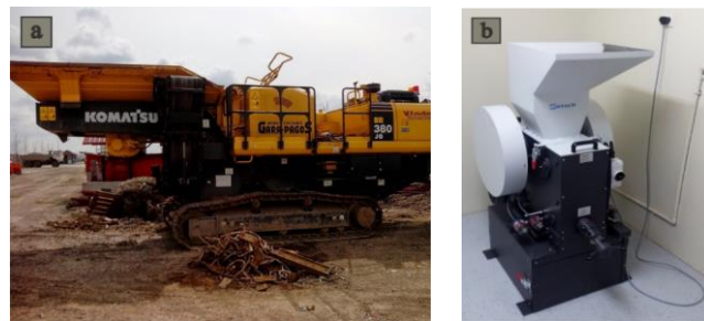
Figure 1. The aggregate crushing process used to transform concrete waste into recycled concrete aggregate (RCA): (a) mobile jaw crusher; (b) laboratory jaw crusher.
