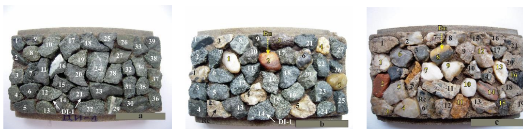
Figure 3. Test samples for PSV with projected ( 38 \pm 2 ) aggregate particles: (a) Dolerite; (b) mixtures 30% RCA (six particles Rc, five particles Ru) and 70% DI-1 (27 particles); (c) RCA.
